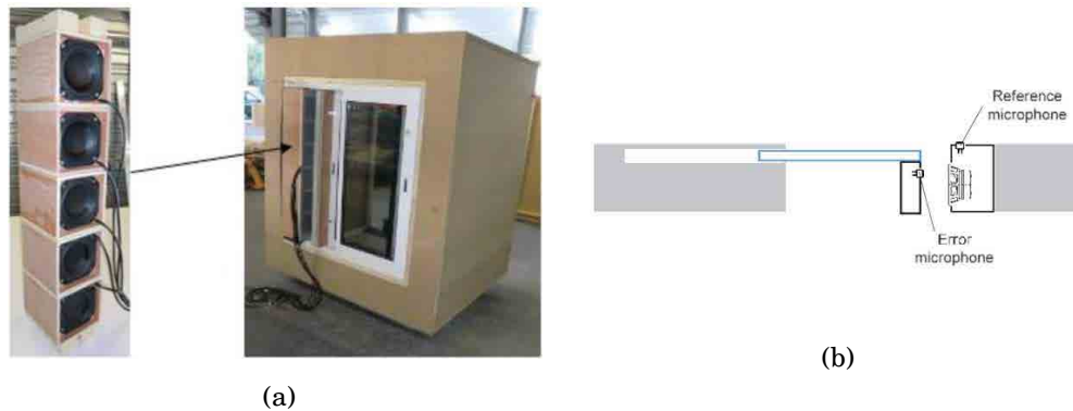
Figure 1.17: (a) Photo of the active window system. (b) The active window with feedforward configuration (Carne et al., 2016).
