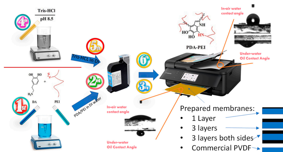
Figure 1. Schematic of the solution preparation and procedure for inkjet printing modification of a commercial hydrophobic membrane. The lower right figures show the schematic representation of the coating configurations of the prepared membranes.
