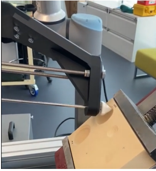
FIGURE 5 Calibration process: using the calibration pointer to touch the surface of acetabulum and select several points. The selected points is used to fit a hemisphere and determine the centre.
