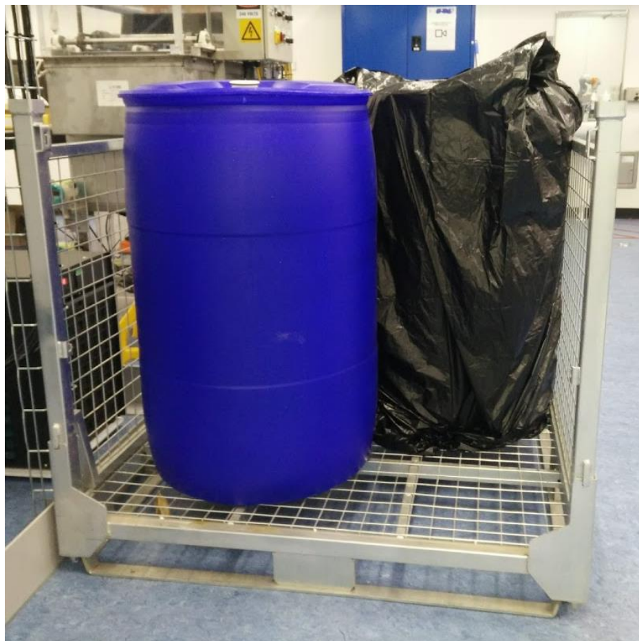
Figure 4.1c After transferring the culture from the bioreactor to 200 litter plastic barrels, the barrels were covered with a black plastic bag to inhibit light exposure.
