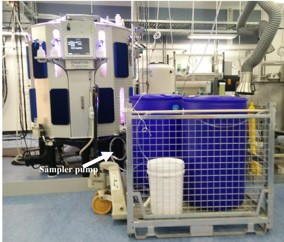
Figure 4.1b Transferring culture from the bioreactor to 200 litre plastic barrels using two way (in/out) sampler pump
