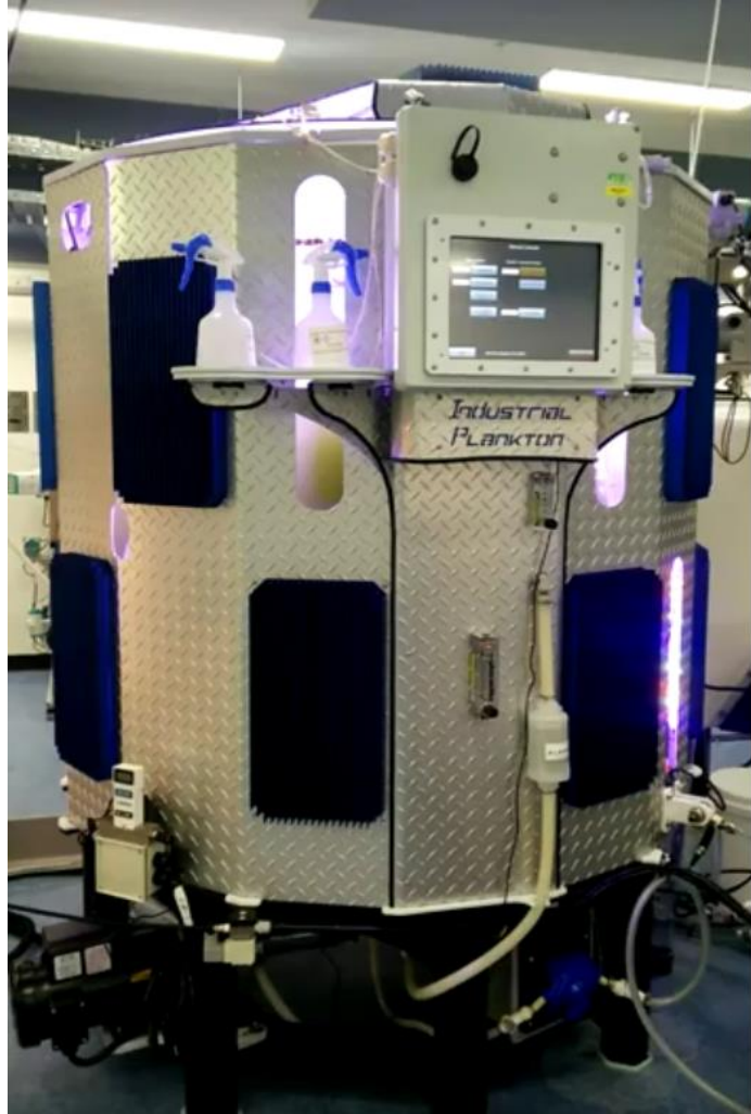
Figure 4.1a 1200-L photobioreactor used for the large scale cultivation of algal biomass to demonstrate the fast settling trait, biomass cultivated in a 12 litres aquarium tanks using nitrogen free BG11. The cultures were mixed with frying pan spoon, image capture after two hours and overnight; to prove the fast settling characteristic of Anabaena circinalis CS-533/02.
