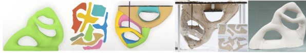
Figure 14: Zhang et al. [ZFS*19] propose a method for the automatic generation of fabric formworks for free-form shapes. The method optimizes the fabric patterns that, once sewn together, will form the flexible formwork for the target shape.
