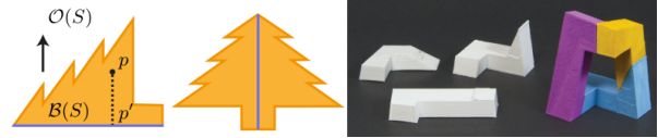
Figure 9: Pyramidality implies the double height field property by definition. This makes pyramidal decompositions [HLZCO14] valid as height field decompositions for the generation of two piece molds.
