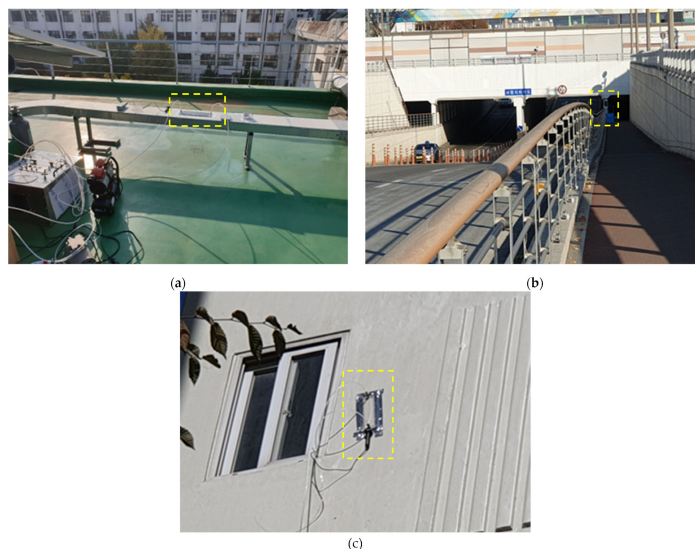
Figure 1. NO x removal measurement locations in real-time at (a) the roof of the building (Gwangju Chonnam University Hall 5), (b) wall of the underpass (West Pyeongju Underground Carriageway, Daegu), and (c) exterior wall of the building (Gerryeo-dong Apartments, Seoul, South Korea).
