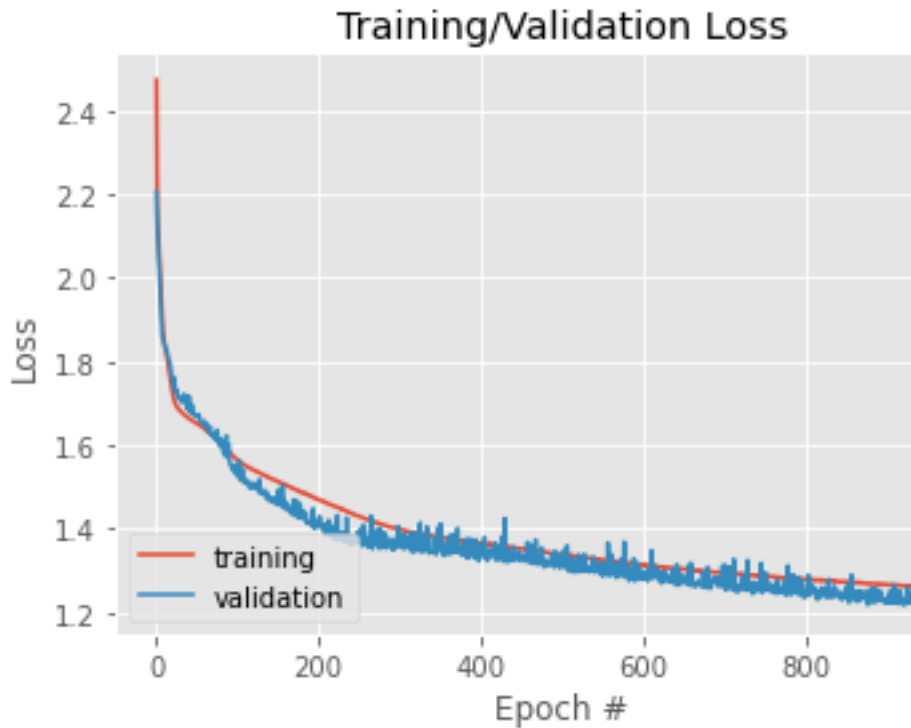
Figure 8(b): Plot of the loss values for the training of the RCNN architecture. Training of RCNN using the Adam optimization configuration and learning rate of 0.00001
