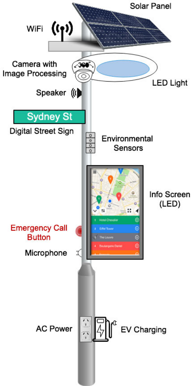
FIGURE 7. Intelligent street light (iLight).
