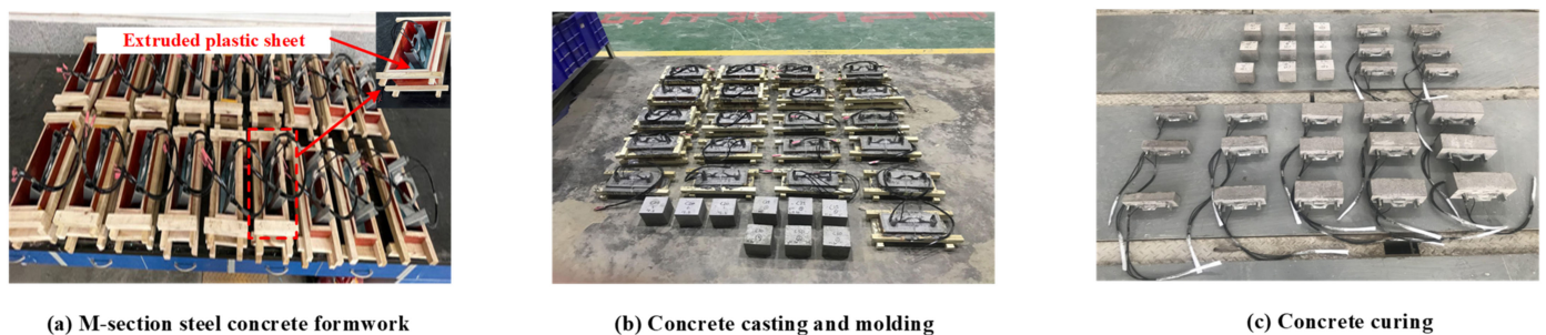
Figure 3. Preparation process of MSSC specimens.
