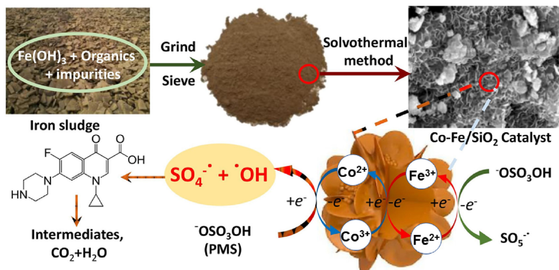
Fig. 5. Waste-derived materials for sulfate radical-based advanced oxidation processes. The preparation of Co-Fe/ \text{SiO}_2 LC and the catalytic mechanisms of PMS [275], Copyright © 2020, Elsevier.
