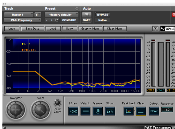
Figure 46: noise floor of recorder only showing a decrease in frequencies above 62Hz.
