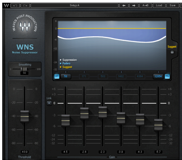
Figure 1 Figure 33: second instance of Waves WNS settings for composition shows further composition reduction.
