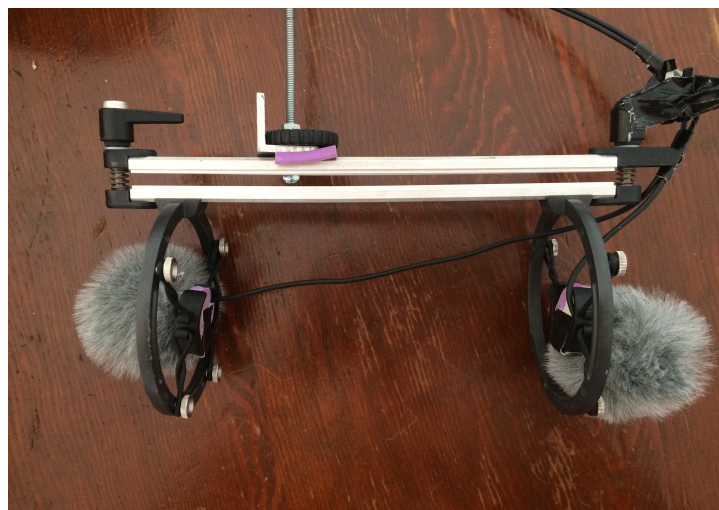
Figure 34: microphones in shock mounts with wind shields.
