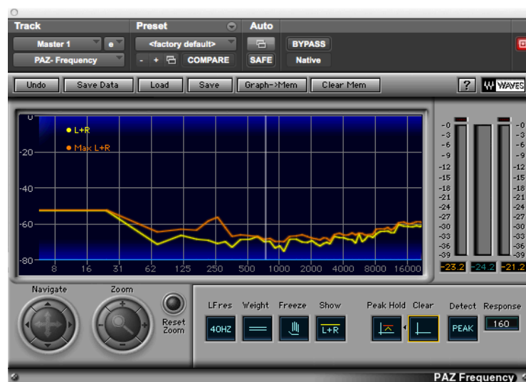
Figure 45: noise floor of adaptors and recorder, removal of microphones presents a decrease between 62Hz – 15Khz, 62Hz and below remains and is identified as noise generated by the recorder as shown in the following.
