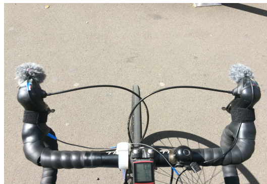
Figure 61: Sanken COS11 microphones set on the handlebars.
