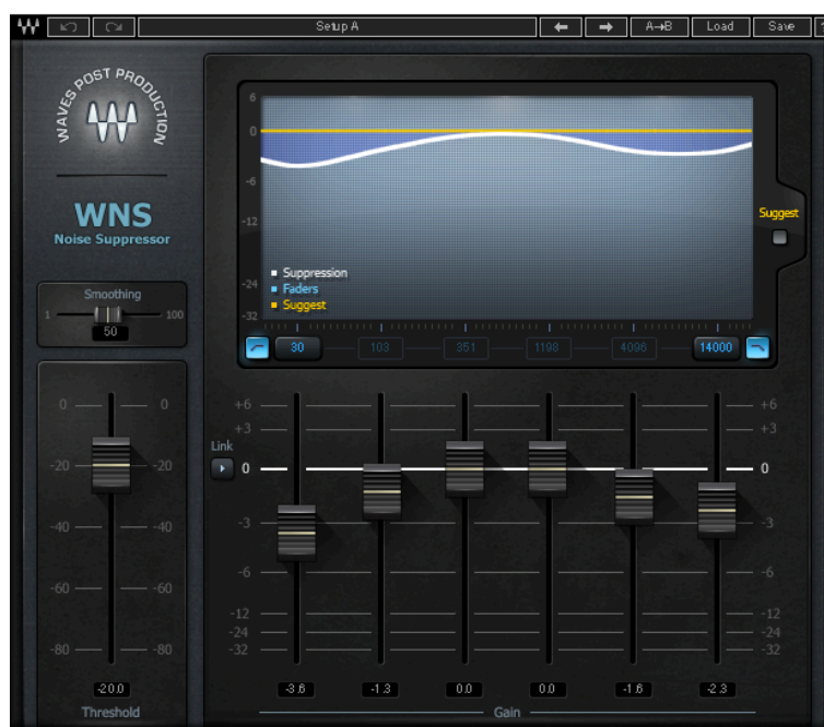
Figure 31: Waves WNS noise reduction settings for sound recordings playback. At this stage noise reduction is used sparingly to remove prominent system noise but ensure to leave the recorded soundscape untouched.
