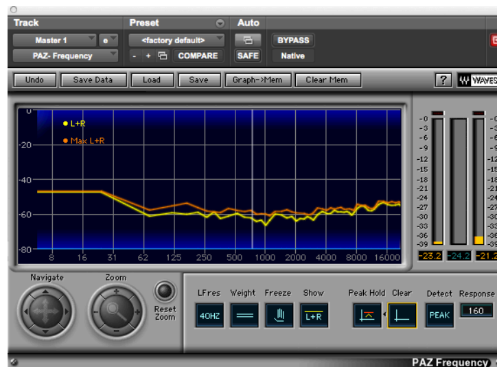
Figure 44: noise floor of microphones, adaptors and recorder.
