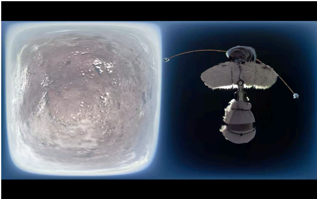
Figure 57: a still from unstitched 360 footage, this is just after burst where the payload is free falling and the camera being flipped, the violent spinning while zooming all the way out created this unexpected image of the payload in one lens and the ground in the other.
