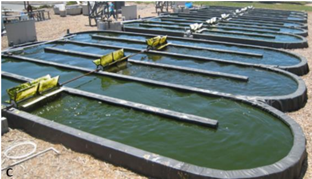
Figure 1-6: Methods of cultivating algae. (A) Bubbled column PBR (B) closed horizontal tubular PBR with pump for mixing (C) Open raceway pond.
