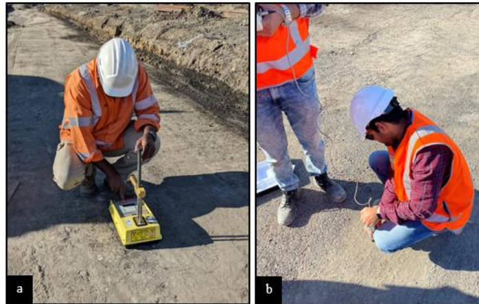
Figure 10. 18: (a) Nuclear density gauge/Non-destructive density Test and (b) the Schmidt Test
