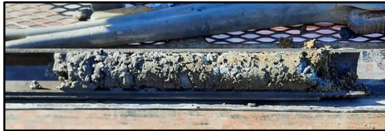
Figure 10. 2: Soil sampling at the instrumented control section (SPT 0-0.5 m)
