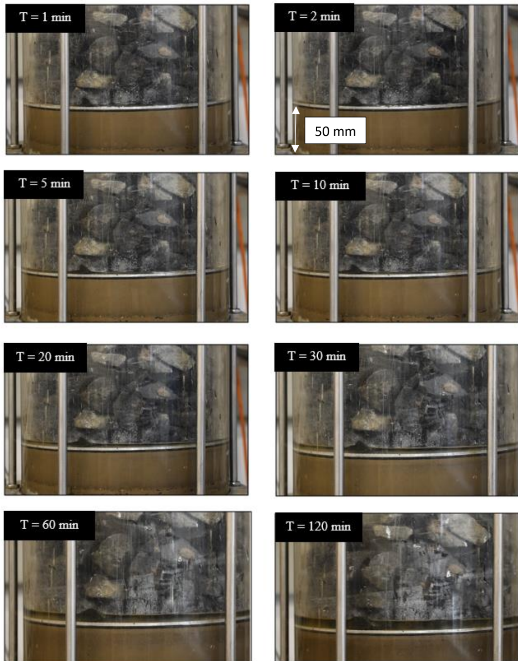
Figure 4. 1: Accumulated water at the top of geocomposite G1
