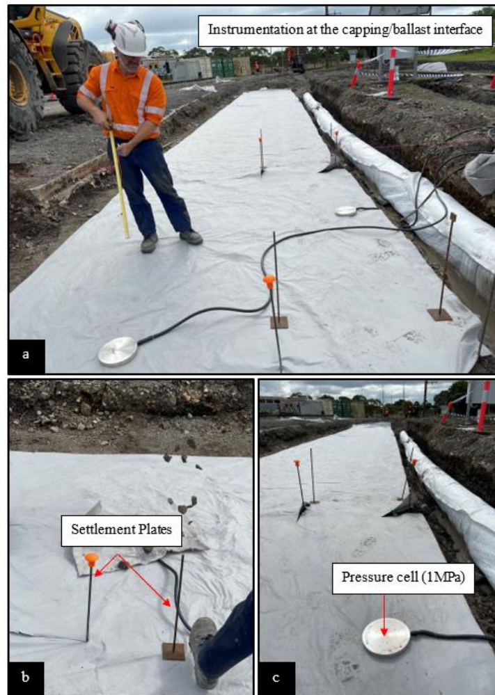
Figure 10. 12: Plan view of ICS instrumentation (a) subgrade/capping interface and (b) Capping/ballast interface (Eng.Analysis)
