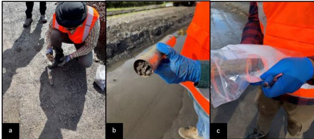
Figure 10. 16: (a) Coring samples at different locations, (b) Cored specimen inside the cylindrical tube, and (c) Extruded specimen for laboratory testing
