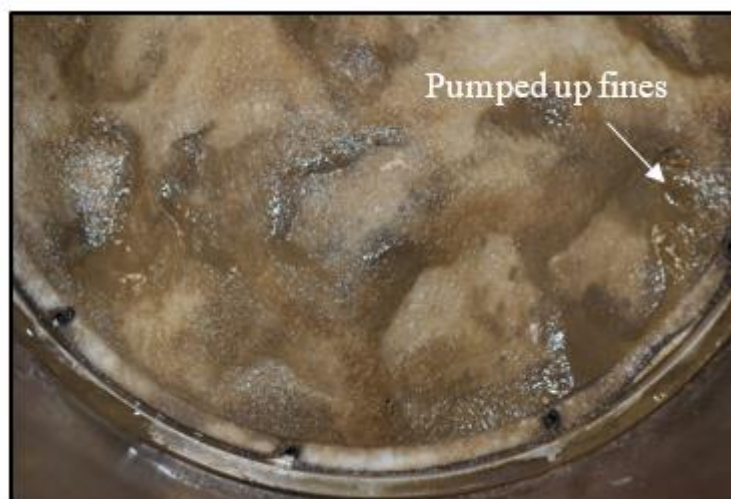
Figure 4. 6: Geotextile G2 after cyclic testing
