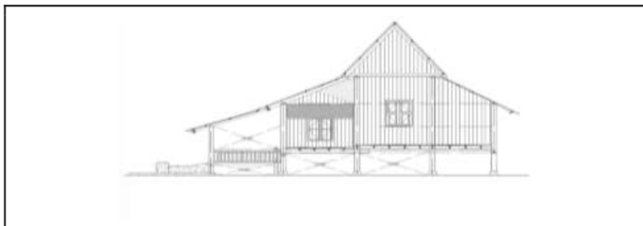
Fig. 9: Section Y-Y of RTAIS, showing the different heights in the veranda and the main house area. (Source: Author, 2022)
