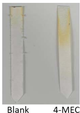
Figure 4-15: Colour change results of the paper-based method included as part of the original study
