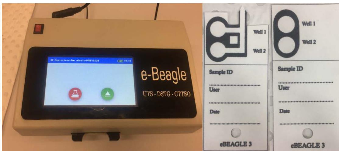
Figure 4-1: e-Beagle device (left) and the two PAD designs which are compatible with the system
