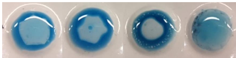
Figure 2-10: Comparison of storage conditions with 8 week old reagent (left to right fresh, fridge, cupboard, laboratory bench)
