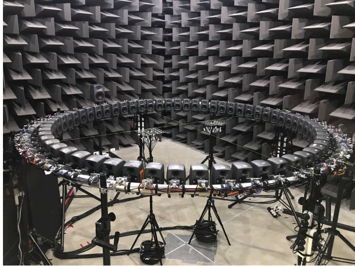
Figure 2 – Photo of the RIRs measurement system with 60 loudspeakers placed along a circular truss.
