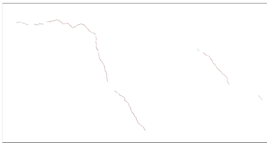
(C) Thinned skeletons of segmented cracks and thinned skeletons of ground truth cracks.
