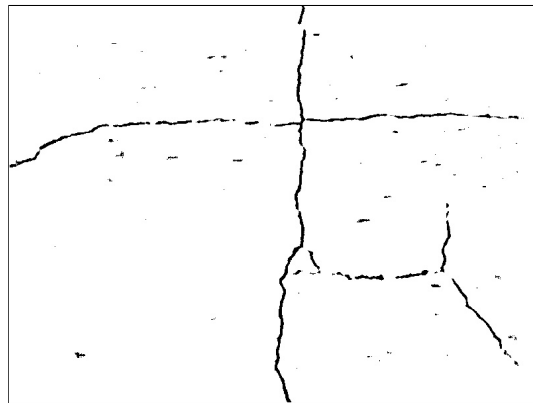
(D) Segmentation result from the combination of Zhang et al. [28] and U-Net [73].
