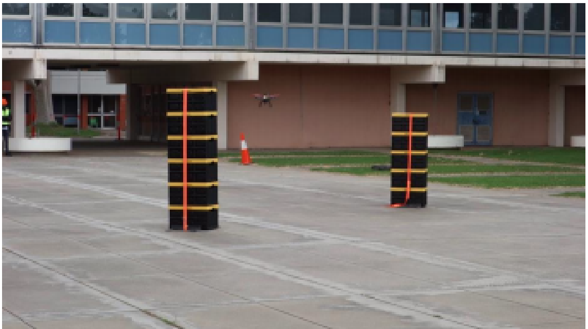
FIGURE A.4: Obstacle avoidance test at the RAAF Williams in Victoria, Australia.
