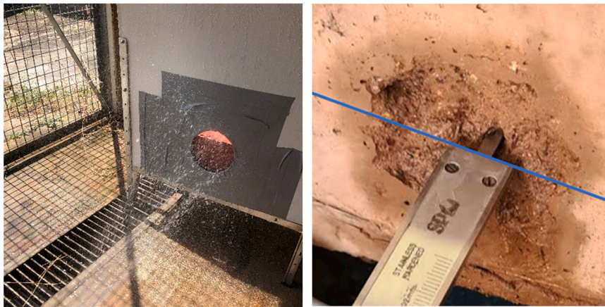
Fig. 6. Left: test setup for accelerated erosion test set up. Right: measuring the pitted depth by using Vernier Calliper.
