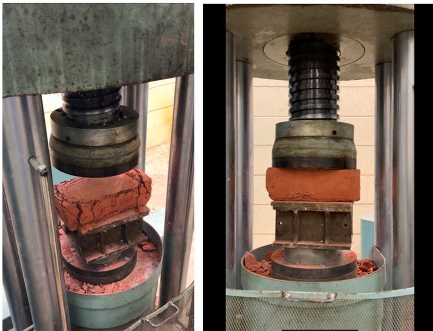
Fig. 4. Mudbricks during and after loading.
