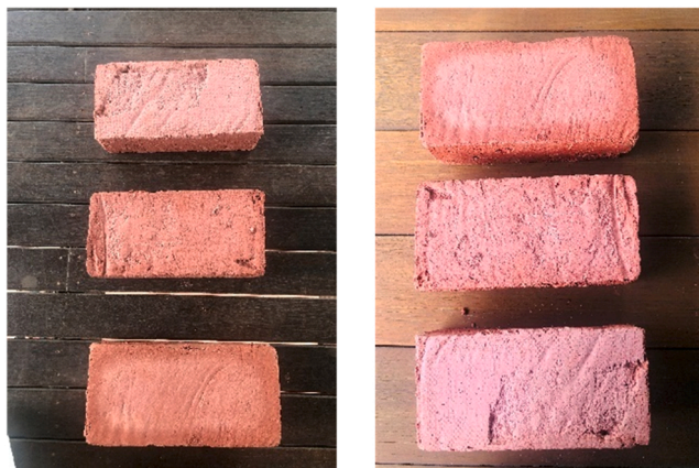
Fig. 3. Mudbricks after removing the moulds.
