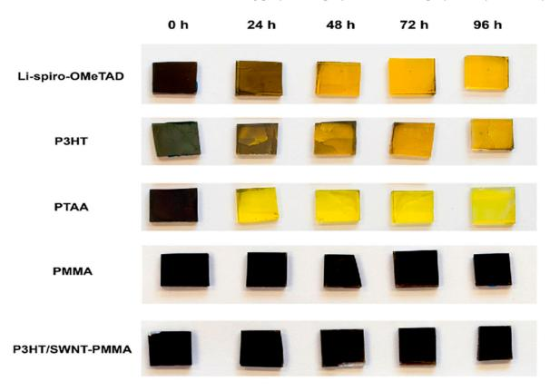
**Figure 3.** Photographs illustrating the visible degradation of the perovskite layer with different hole transport layers exposed to 80 °C under ambient conditions. The conversion from the dark initial color to yellow indicates the degradation of the perovskite material to lead iodide. Over 96 h of heat exposure, only a composite structure of carbon nanotubes and PMMA was able to prevent degradation. Reprinted with permission from Ref. [114]. Copyright: American Chemical Society 2014.
