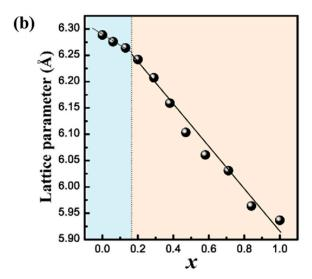
**Figure 4.** (a) Power conversion efficiency of the MAPb( $I_{1-x}Br_x$ )<sub>3</sub> (x = 0, 0.06, 0.20, and 0.29)-based solar cells measured in the air (at room temperature) without encapsulation; and (b) the lattice parameters of pseudo cubic or cubic MAPb( $I_{1-x}Br_x$ )<sub>3</sub> as a function of Br composition (x). Reprinted with permission from Ref. [157]. Copyright: American Chemical Society 2013.
