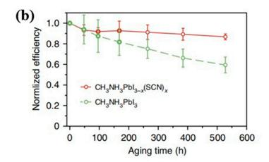
**Figure 5.** (a) Images of different  $(CH_3(CH_2)_3NH_3)_2(CH_3NH_3)_{n-1}Pb_nI_{3n+1}$  perovskite films before and after exposure to 40% humidity (Reprinted with permission from Ref. [159]. Copyright: American Chemical Society 2015); and (b) the evolution of the PCEs of  $CH_3NH_3PbI_3$  and  $CH_3NH_3PbI_{3-x}$  (SCN)<sub>x</sub>-based solar cells after gaining in air without encapsulation (Reprinted with permission from Ref. [58]. Copyright: Springer nature 2016).
