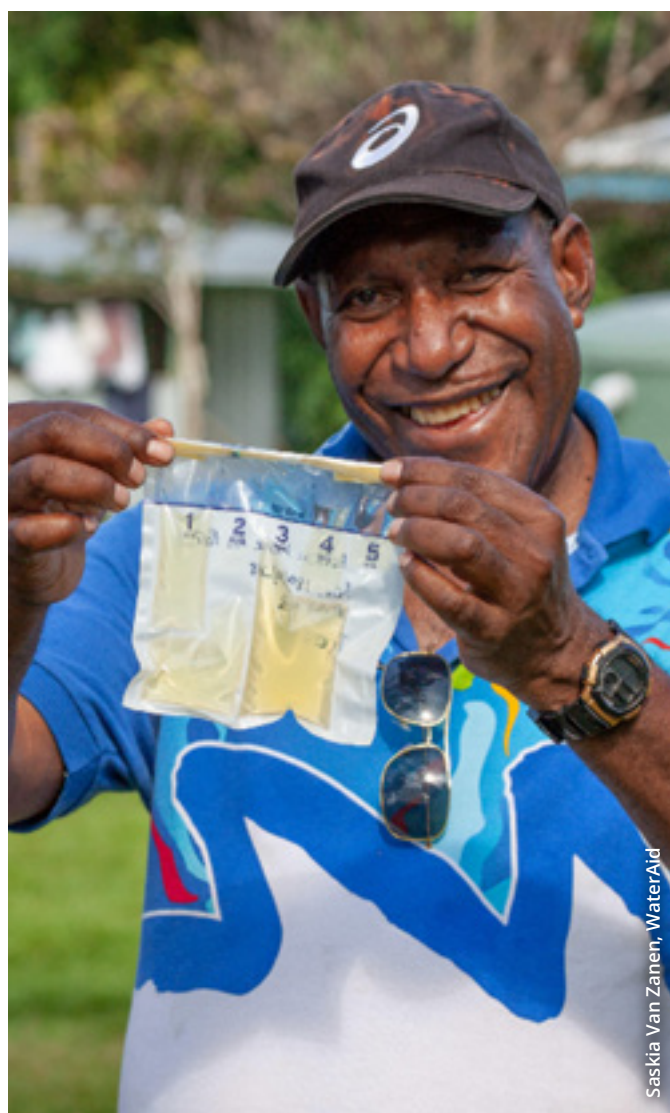
Figure 26. Wewak Islands LLG Manager Mr Gideon Kavi takes a water quality sample using the Aquagenx CBT.
