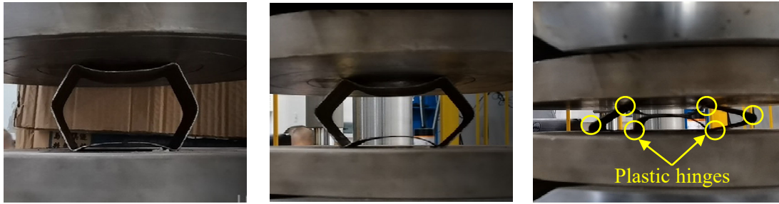
Fig. 19. The deformation of the rectangular steel tube
