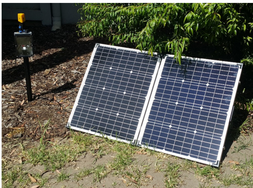
Figure 6. Camera trap setup consisting of camera trap mounted on stake, recording the ground, and solar panel powering the setup.
