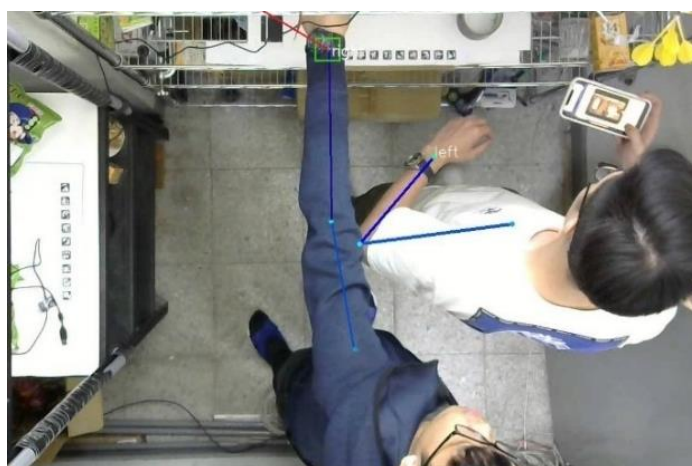
Figure 5. Using OpenPose to determine the purchase status of customers.
