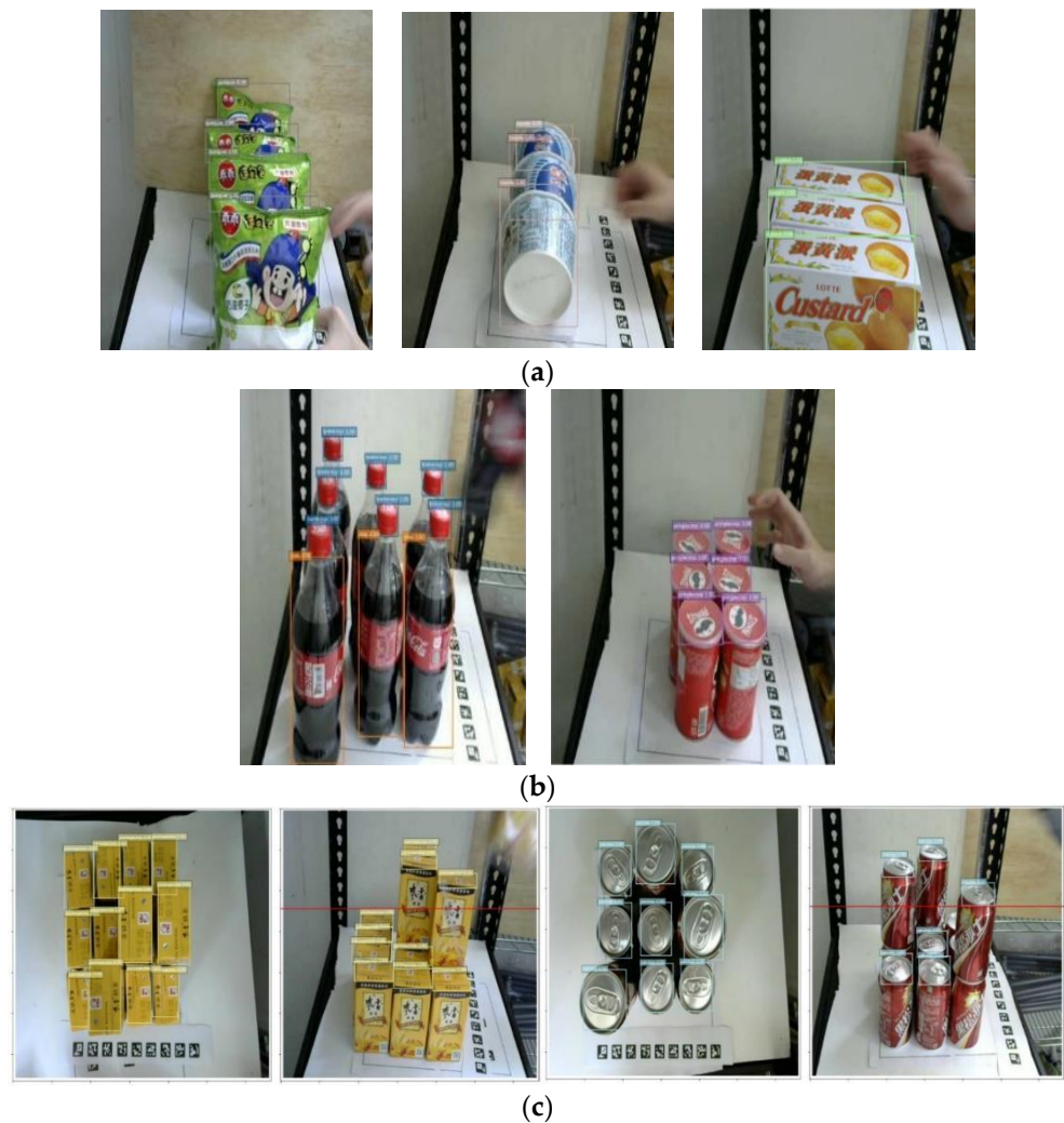
Figure 10. Identifying products in different categories. (a) Packed products; (b) top view for dense products; (c) top and side views using two cameras.
