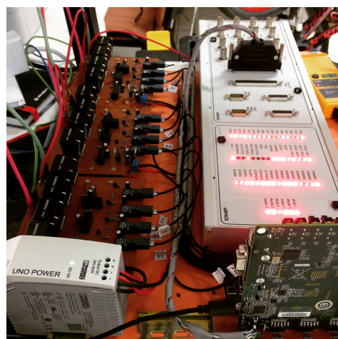
Figure 10. Implementation for a 27-level asymmetric multilevel converter.
