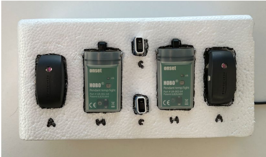
Figure 2.2: Apparatus used to simultaneously collect light intensity from three pairs of different LDLs.
