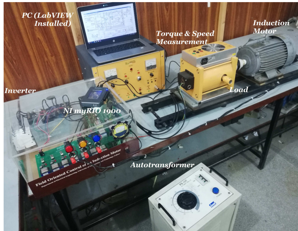
Figure 10. Induction machine drive testing platform.
