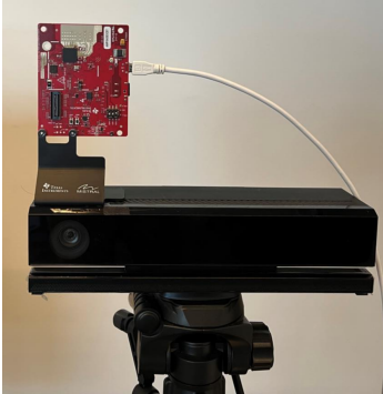
Fig. 3: Mmwave radar and camera
