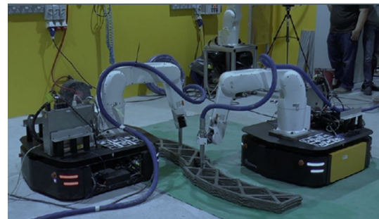
Fig. 8 Collaborative mobile robots building a wall structure (Zhang et al. 2018)
