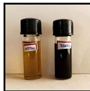
Fig. 1. Synthesis of silver nanoparticles using propolis extract (AgNPs). The color change from yellow to dark brown between the initial and final stage of synthesis.
