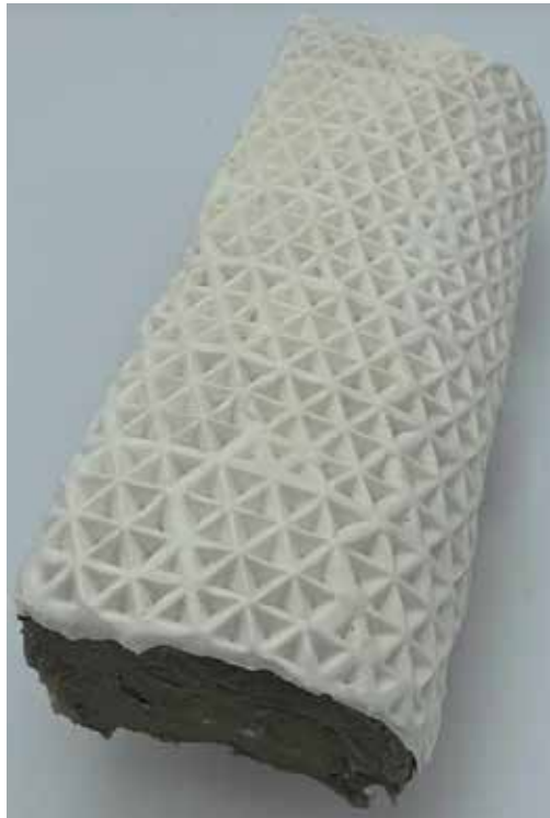
Figure 5. Multiple internal cube corners surface texture prototype.
