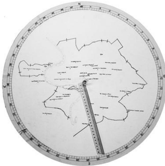
Figure 2-1 - A Reproduction of Alberti’s Horizon Instrument. (Nasifoglu, 2012)
