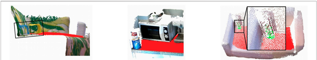
FIGURE 8 | Examples of missed objects. Extracted planes are visualized in red. First image: two objects in black rectangle. Only the yellow cup is detected because the couch seat is too curved. Second and third image: only few object points are within the convex hull of the plane and therefore classified as noise and rejected. Note, that in the third example the reconstruction is very sparse because the robot did not get close enough to the surface.
