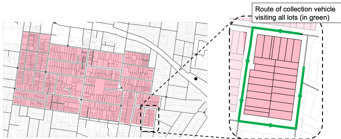
Figure 5-8: Overview of the approach used for estimating the between-bin collection travel in the kerbside collection component of the waste collection and transport model
