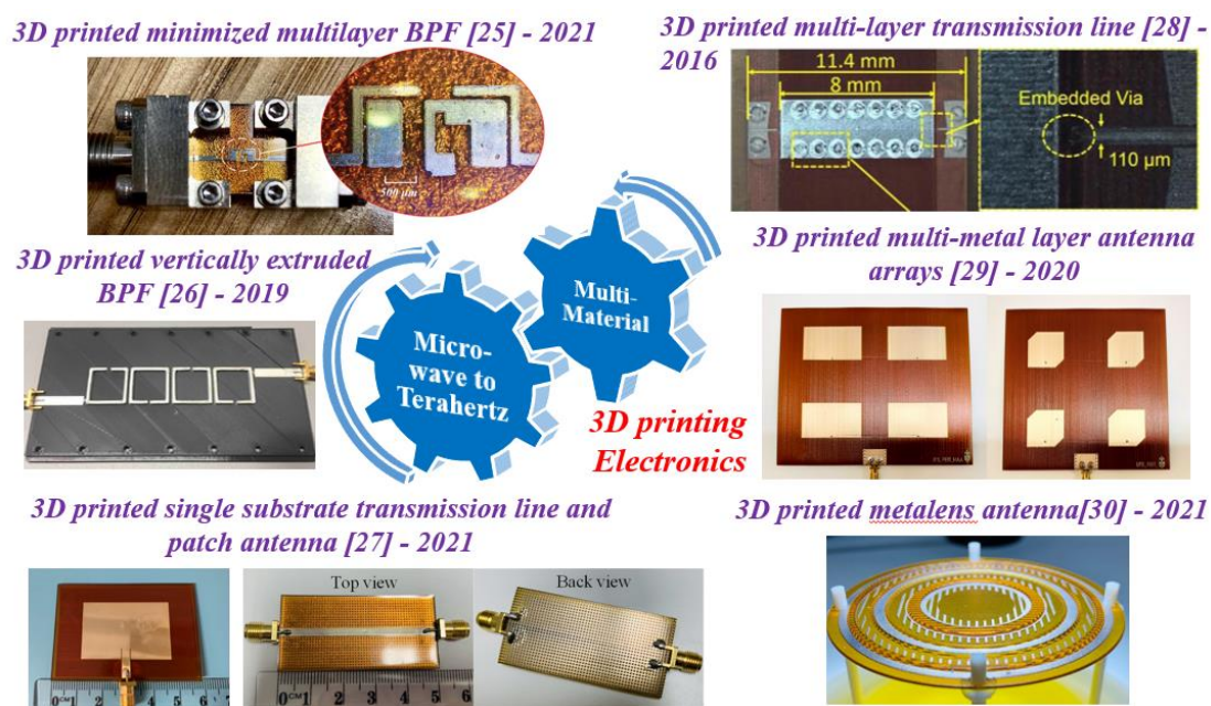
Fig. 2.1. Emerging 3D printing technologies in microwave components and radio frequency electronics - a game changer in the manufacturing value chain in Industry 4.0.
