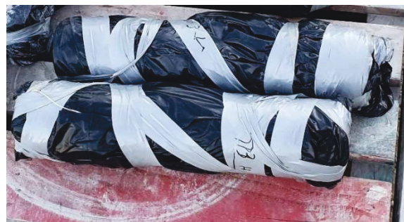
Figure 5.1 Push tube sampling (a) push tube being pushed into landfill by 20 tonne excavator, (b) sketch of custom made push tube and (c) sealed push tube samples
