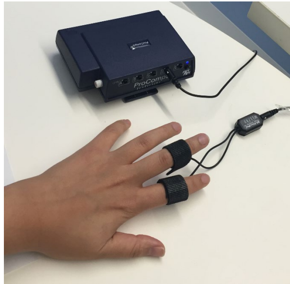
Figure 2.5 illustrates the attachment of the skin conductance sensors to the medial phalange of the middle and index fingers of the non-dominant hand of the subject.
