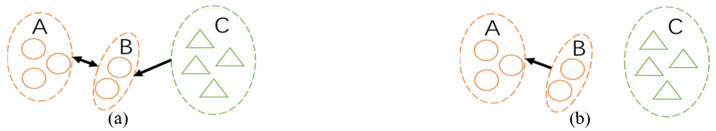
Figure 5.1. a simple example of the traditional NNC merging process (a), and the CNNC procedure (b). We employ dotted lines to denote clusters (i.e., A, B, and C), and circles or triangles to represent data samples. In traditional NNC, cluster A and cluster B are chosen to merge, cluster C and cluster B are chosen to merge, because cluster A and cluster B are the nearest neighbor of each other, and the nearest neighbor of cluster C is cluster B. However, in the CNNC, cluster C and cluster B are not chosen to merge because \text{mass}(C) > \text{mass}(B) .
