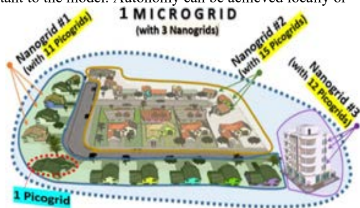
Figure 60: A microgrid with 03 nanogrids and 38 picogrids
