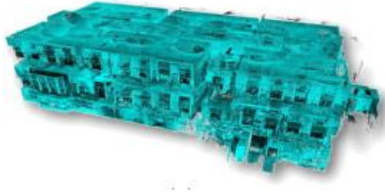
Figure 2.3: 3D as-built reconstruction of a building using point cloud
