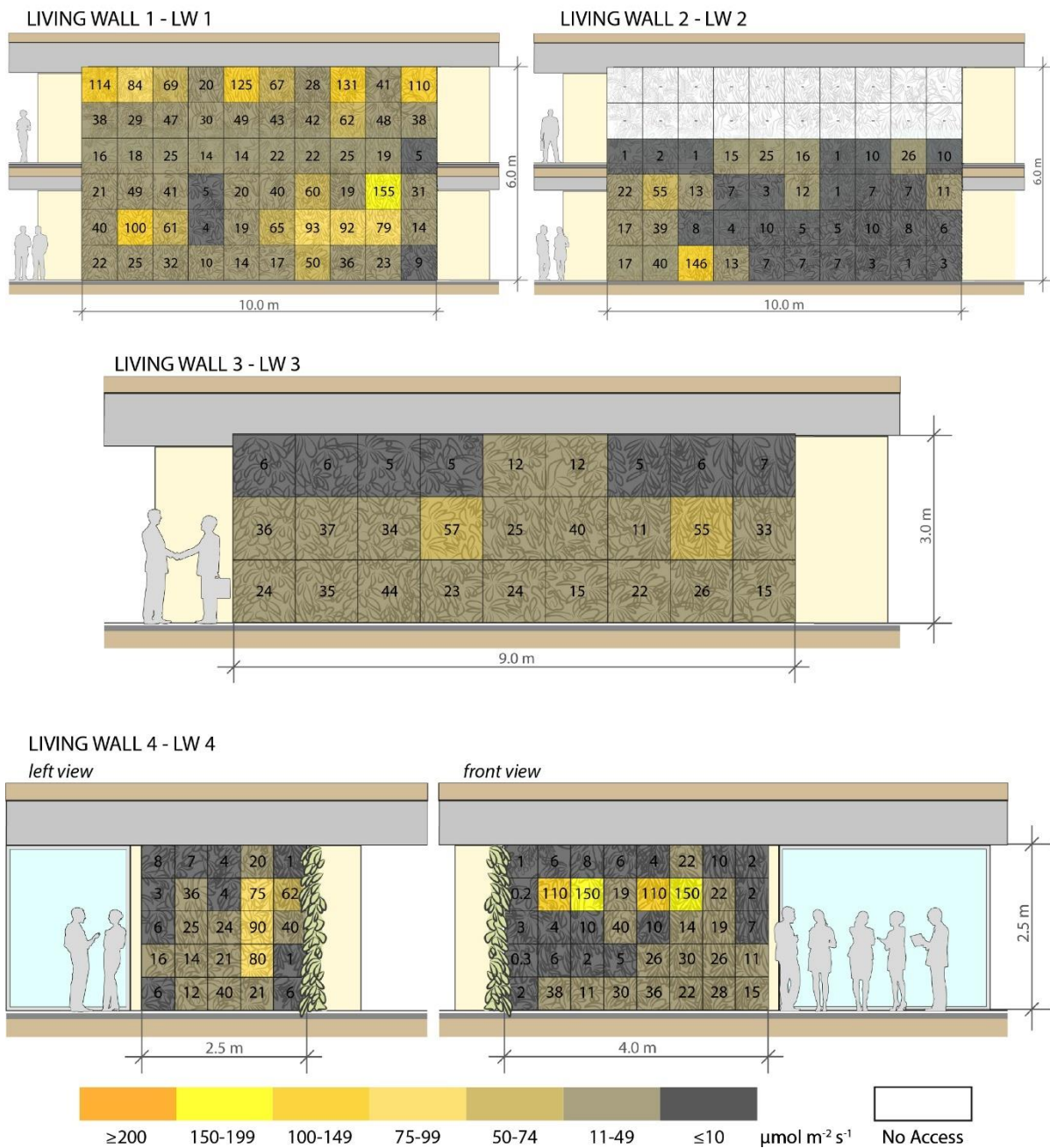
Figure 4. Lightmap of the four Living Walls (LW 1 – 4). Light measurements were taken at 1 m intervals for LW 1-3, and at 0.5 m intervals for LW 4 due to the relative complexity in both design and plant composition. The number within each square represents the average light intensity ( \mu\text{mol}\cdot\text{m}^{-2}\cdot\text{s}^{-1} ) available at the plant canopy for each 1 m 2 area of living wall (0.5 m 2 for LW 4). No access was available for light measurements at LW 2 for the upper 20 m 2 due to infrastructure limitations.
