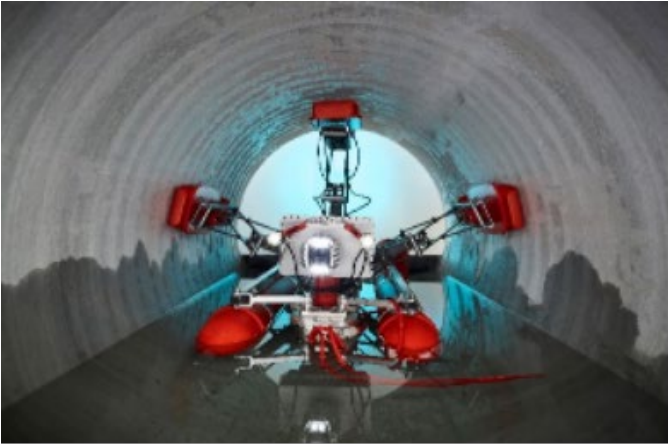
Figure 4: CRAFT V1 with scissor lift expansion arms to handle sensor payload, 100m Cable reel with power and communication to CRAFT.
