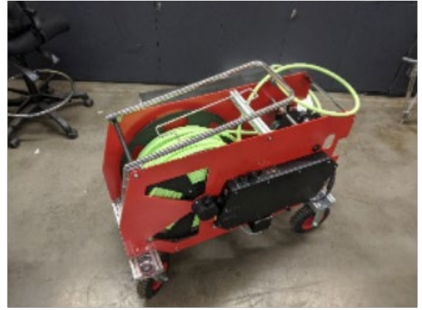
Figure 4: CRAFT V1 with scissor lift expansion arms to handle sensor payload, 100m Cable reel with power and communication to CRAFT.
