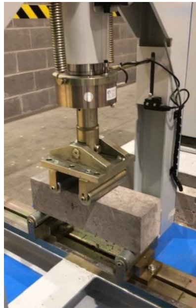
Figure 3-11 Set up for modulus of rupture test
