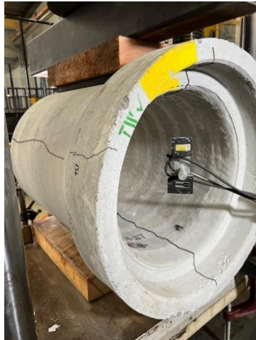
(b) Flexural cracks in pipe
