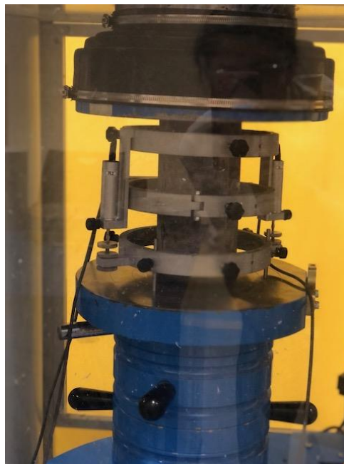
Figure 3-13 Test set up to determine Modulus of Elasticity of concrete
