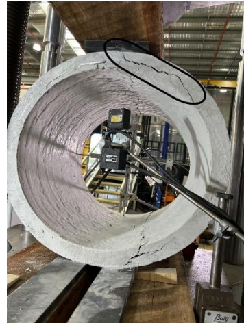
(c) Radial tension cracks
