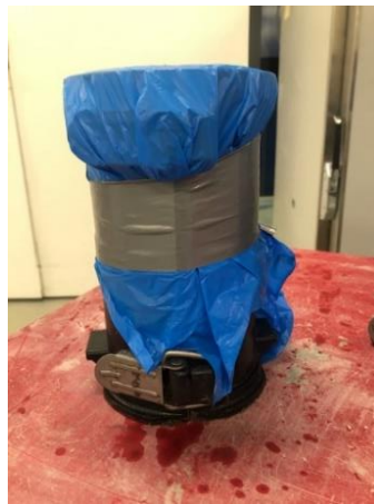
Figure 3-4 Concrete cylinder sealed before heat curing
