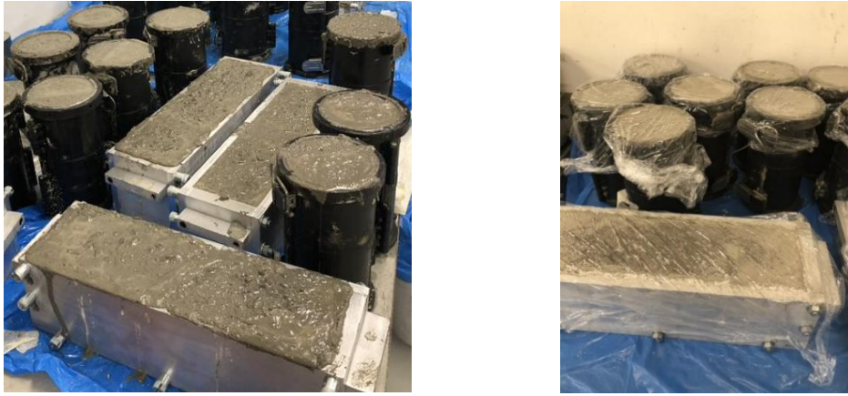
Figure 3-3 Concrete cylinders and beam casting
