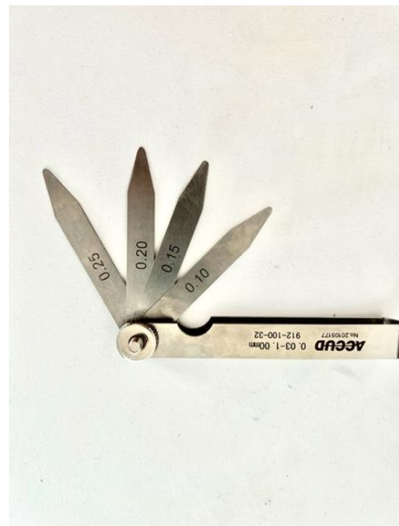
b) Feeler gauge to measure crack
