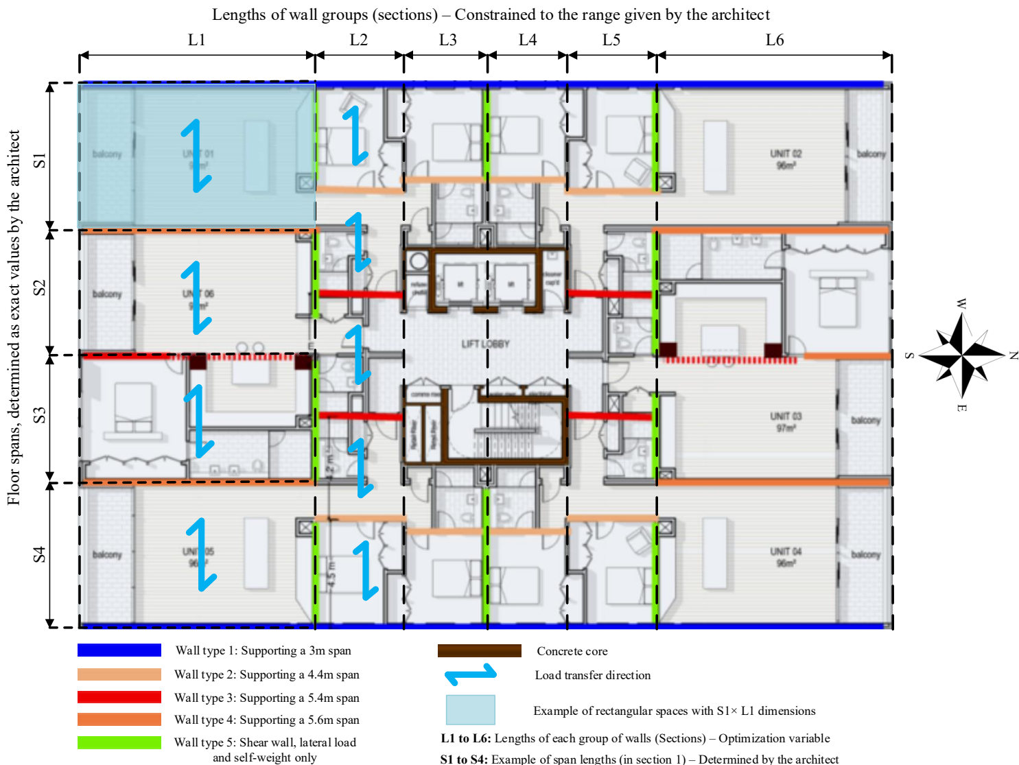
Figure 5.2: Example floor plan with a one-way spanning floor system (adopted from Woodard and Jones [162])
