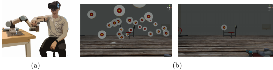
FIGURE 2.12: (a) A system based on the GAVRe2 framework. (b) First-person view from inside VR [11].
