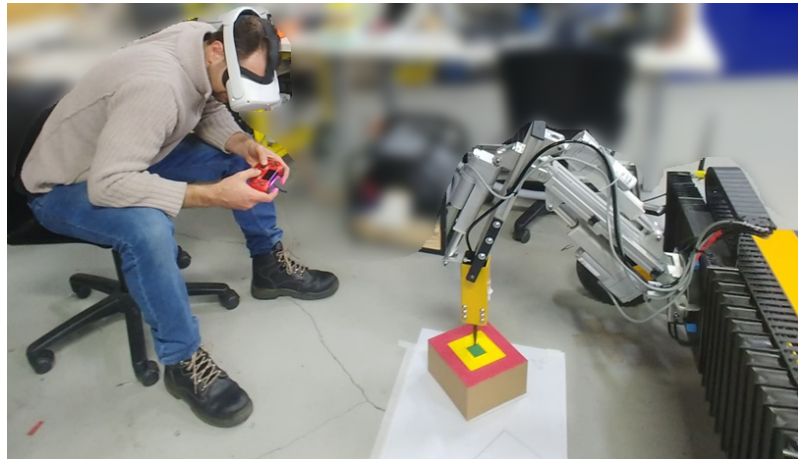
FIGURE 6.9: A participant manipulating the end-effector to the green area of the target while in VR.
