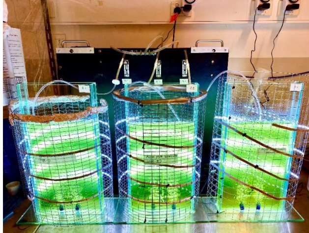
Figure 56: A photo of batch-mode microalgae reactor.
