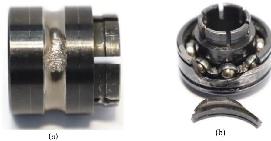
Figure 4.4. The failure bearings: (a) Inner race wear (b) Outer race fracture [148]
