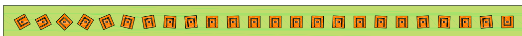
Figure 4.8: The 24-element rotated U-slot loaded patch antenna array obtained in the flat-top shaped pattern synthesis case.
