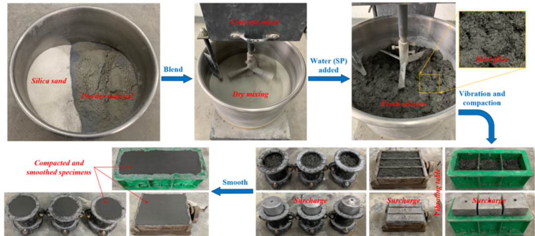
Fig. 3.2. Preparation process of FR-DUHPC samples for static mechanical tests.
