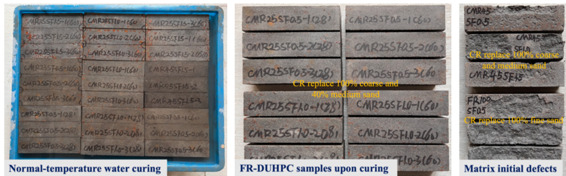
Fig. 5.2. Water curing and typical FR-DUHPC samples containing CR aggregate.
