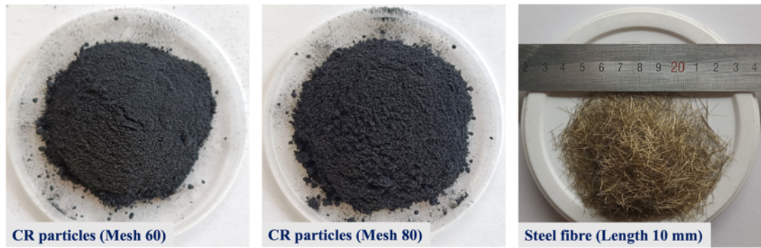
Fig. 5.1. Appearance of silica fume, FA, GGBS, CR particles and steel fibres.
