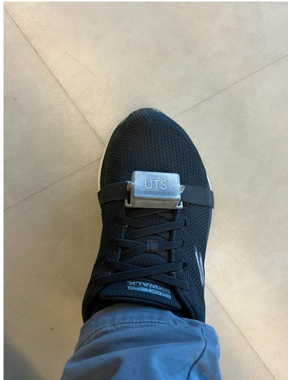
Figure 4.4. IMU sensor placement on the foot
