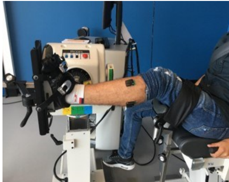
Figure 4.7. Ankle torque data collection using an isokinetic dynamometer
